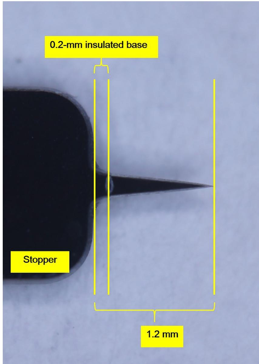
Figure 3 / S type needle used for the procedure. The length is 1.2mm and the shoulder of the base part acts as a stopper to prevent the needle from getting too deep into the skin. Since 0.2mm from the base part is treated with insulation coating, the epidermis is protected.
